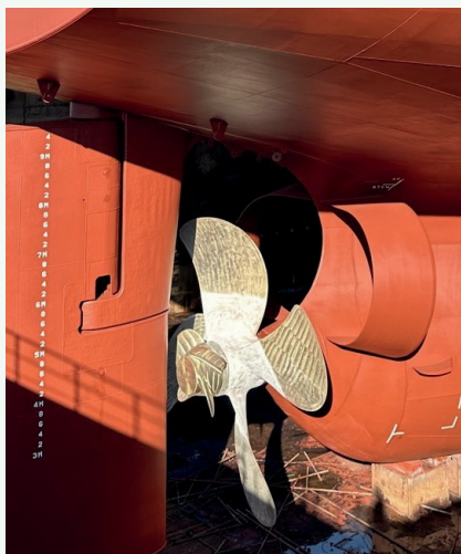
Wake Equalising Duct and PBCF
